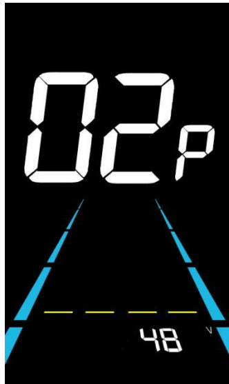
Figure 6-2 Rated voltage setting interface
