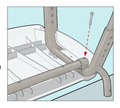
4. Place the Left Leg onto the seat, capturing the Cross Bar in the Bracket. Secure the Legs with the remaining Short Screw and Long Screw as shown.
