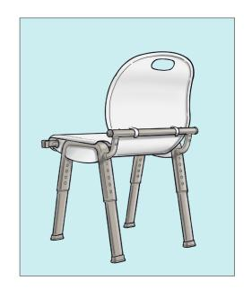
3. Tilt the chair forward and attach Seat Back to Cross Bar using included Long Screws and Allen Wrench.
