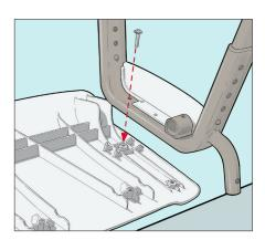
3. Place the Cross Bar into the Cross Bar Bracket so that the holes in the Bracket and Cross Bar lineup. Place a Long Screw through these holes, then screw it into the Seat using the supplied Allen Wrench. Do not fully tighten the screw yet.
