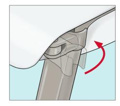
7. Attach the Towel Bar to the back support tubes. Orient the Towel Bar so the spring pins face the back of the chair, press the spring pins, then insert into the support tubes. Make sure the spring pins click into the holes on the support tubes.
