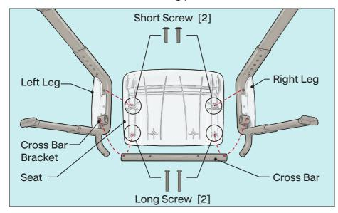
Orient the parts as shown above. Note that the height adjustment holes on the Legs should face the back edge of the seat. The plastic side panels on the Legs should be facing outward and the Cross Bar Brackets should be facing inward. There are 6 mounting points for screws on the bottom of the seat. This part of the assembly will use the 4 identified above with the noted hardware.
