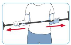
1. Grasp the bottom shaft section and top shaft section. Pull away from each other, exposing the hinges.
