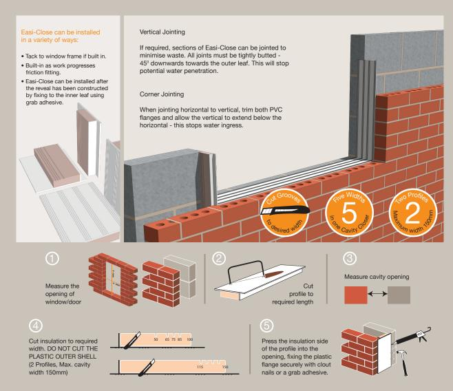
Two profiles available to fit: 50-100mm cavities & 100-150mm cavities
