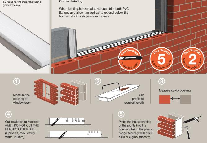
Two profiles available to fit: 50-100mm cavities & 100-150mm cavities
