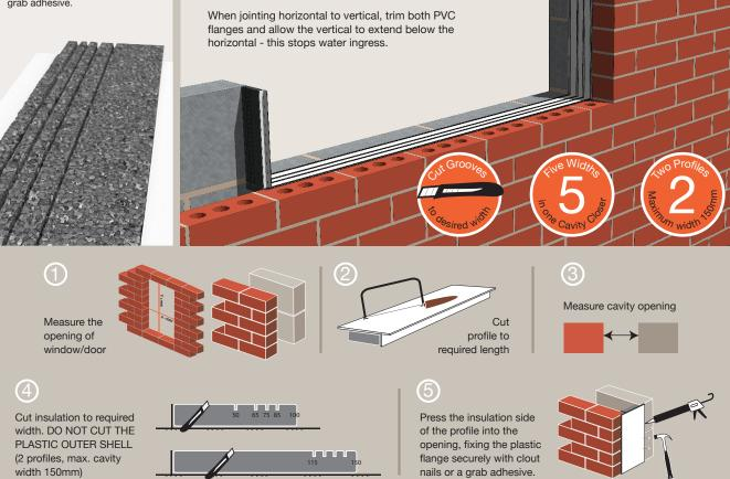
Two profiles available to fit: 50-100mm cavities & 100-150mm cavities
