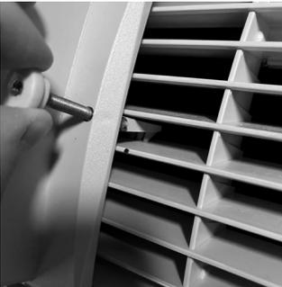
4. Slide clamp into the vent until it grabs the bottom of the vent.
