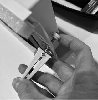
1. Remove the existing clamp from the center frame by removing the nut.
