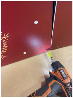
2. Remove the four screws from the center panel to remove the graphic (to be reattached later).
