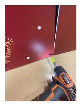
5. Once all bolts are secure, reattach the center panel graphic using the provided self-tapping screws.
