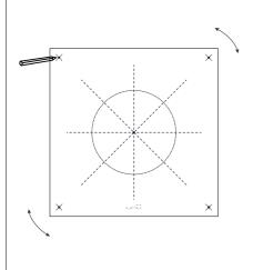
2. Drill all marked points and use the appropriate wall plugs (not included). Place the L shaped hook screws on the wall, distanced about 25mm from the wall, facing up or down, as displayed in the illustration.
