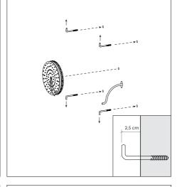
**3.** Fix the LED support to the wall with the provided screw (it is necessary to use a M8 wall plug - not included). Cut the electrical cable leaving around 25cm.
