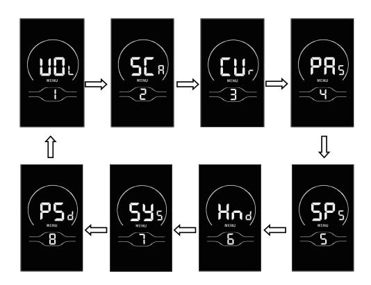
Select the settings via  $\ +\ /\ -\$  and press  $\ i\$  to enter the corresponding setup windows.
