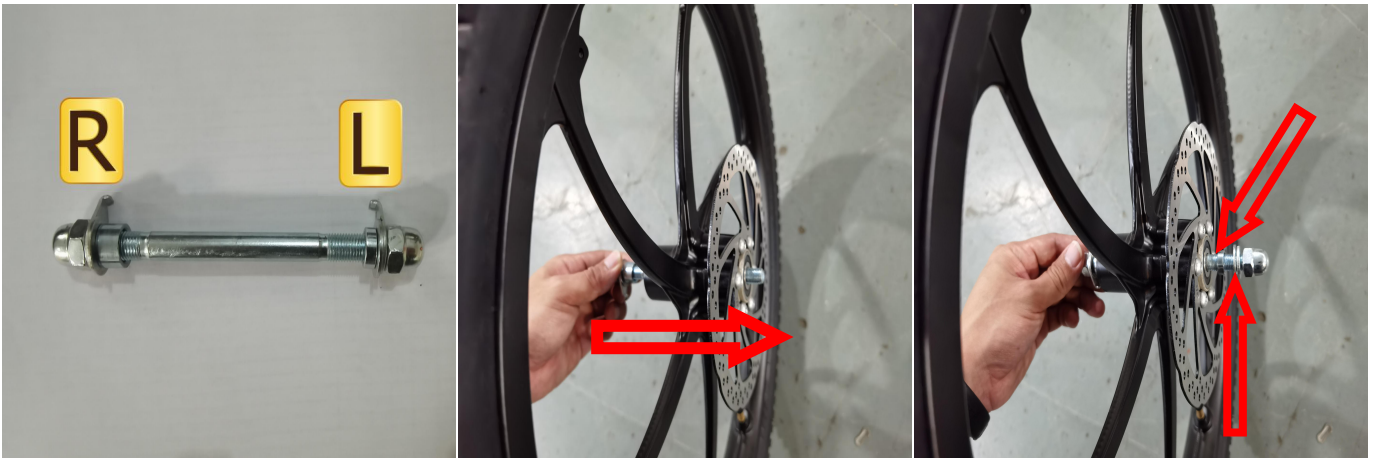
3. When the front wheel is mounted on the fork, the washer is on the inside, and a gasket is added on the outside and a safety hook is added.
