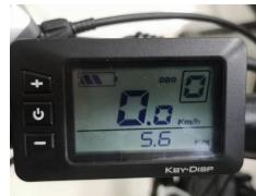
To switch on/off the E-Bike system, hold the button for 2s. The system default value is "1" low speed. (Pure electric mode+ assist mode)
