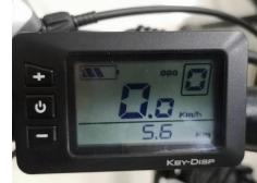
To switch on/off the E-Bike system, hold the button for 2s. The system default value is "1" low speed. (Pure electric mode+ assist mode)
