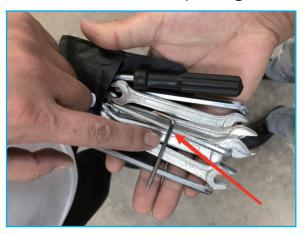
1.5 Open the meter clamping screw with 3# Hex key wrench anticlockwise.
