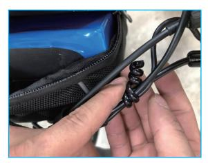
1.3 Unplug the meter line's butt connector.
