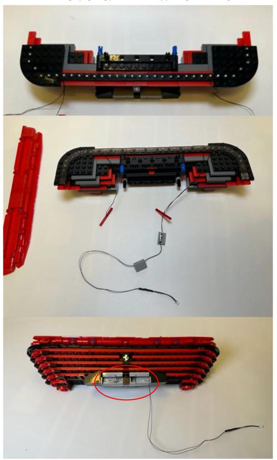
Before putting the rear part back to the car, make sure the connector is on the top and the red lighting bars go to the bottom
