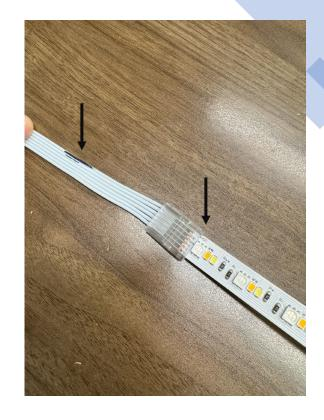
Confirm that the VDC24+ should be lined up to the black marker indicator.
