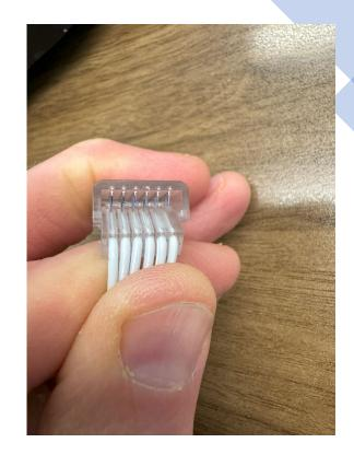
The pins will push into the wire making contact with the copper inside.
