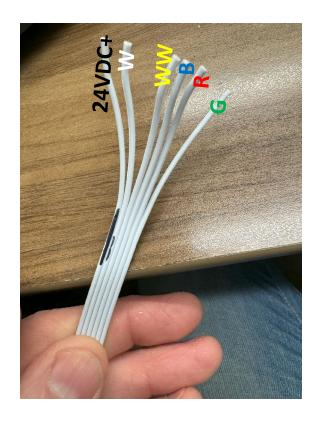
Repeating the process from earlier, spread the wires apart. Note the wires must match up from the other side when connecting to the second piece of tape.
