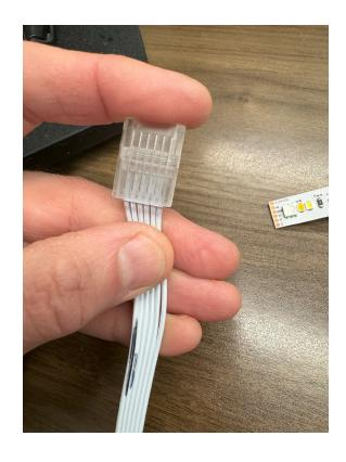
Clamp down by hand or with wire pliers to secure.
