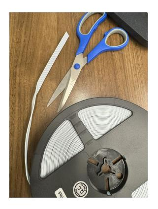
Cut the 6-pin wire to desired length.
