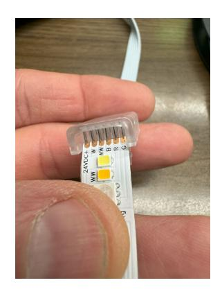
Take the cut end of the tape and insert so the pins in the connector contact with all 6 copper markings.
