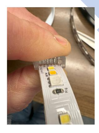
Press together to secure, you may use wire pliers or another tool to secure.
