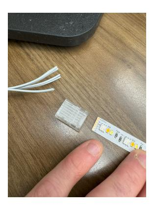
Stage the 6-pin wire, the wire-totape connector and the beginning of the next tape run. Make sure the 24VDC+ lines up with the right wire and the connector contacts will line up properly with the copper markings.
