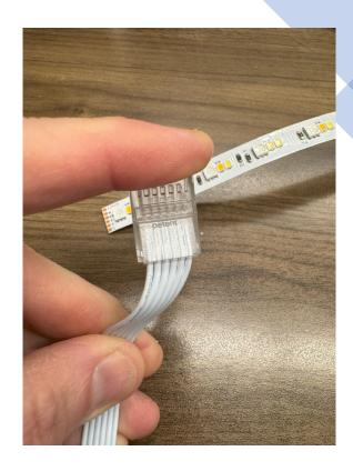
Insert the wires in the holes, again making sure that they are not tangled.
