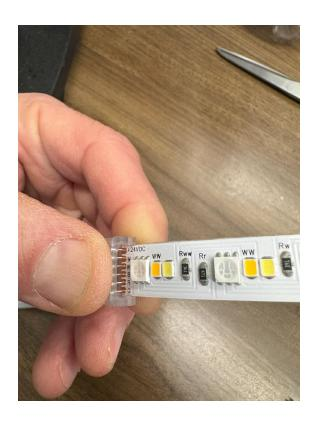
Line-up the copper marks to the pins of the connector and clamp down.
