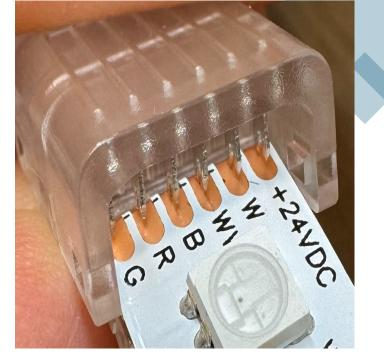
Prior to installation, make sure the tape is cut at the copper indicators. The markings of the tape must match up.
