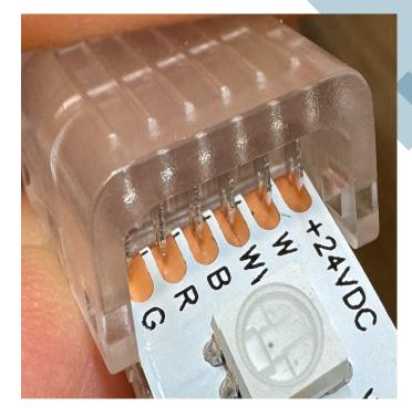
Make sure the connector is lined so the connector pins press down into the copper indicators on both ends. Use pliers, or another tool, to secure each end of the connector.
