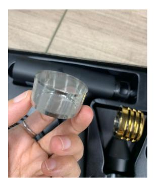
D. You can then put it back as well as the gold piece. Make sure direction is right when you try to rotate back in. The side which has space in between is supposed to be on the top. You can refer to pic 1 above.
