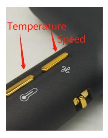
Tips 2: you can remove the back cover (gold part) to clean the air inlet section, which will make sure air goes in smoothly, to keep a longer life of the motor and dryer.
