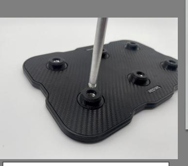
2. SCREW IN ALL 6 RODS INTO THE BASE FIRMLY
