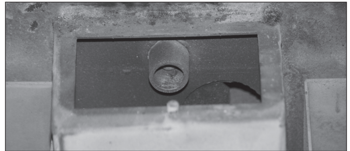
Figure 35: Remove ash from igniter tube (underneath firepot)
