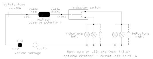
Attention! The minimal supply cable width is 0,75mm<sup>2</sup>. You must fuse the +12V power supply cable with a 10A safety fuse. If the device will be used without fuse, damage at the connecting cable or the mo.flash itself can cause a shortcut and a cable fire. There may be a risk of your life! If you are not capable to connect the device properly, let the professional motorcycle technician do the job.
