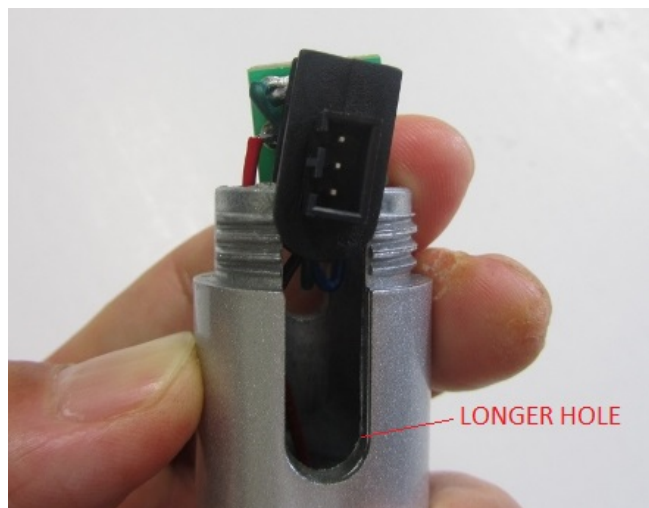
[Picture 15: Insert Switch & 3 Pin Module]
