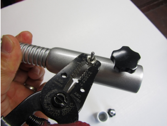
[Picture 6: Remove nut from switch]
