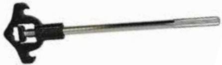
K05 Adjustable Hydrant Wrench (Double) For pentagon heads up to 1 7/8" and square 1 1/2" - Double hook spanner head fits 3/4" to 6" rocker lug or pin lug fittings -Replaceable jaw
