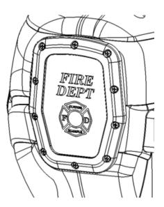
**Warning:** Over-tightening these screws may damage the Light Modules requiring replacement. Damage caused from over tightening is not covered under product warranty.
