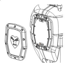
3. Remove the 'Elk & Heart' logo lens from the bezel as shown. Install the custom lens into the bezel. Ensure that the bezel O-ring is still seated in the bezel. Reinstall it if it has fallen out of place. The custom lens should be installed so that the coated side will be on the inside of the light module assembly once reattached to the assembly.
