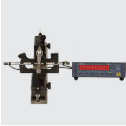
Measuring a shaft with 2 probes (A+B)
