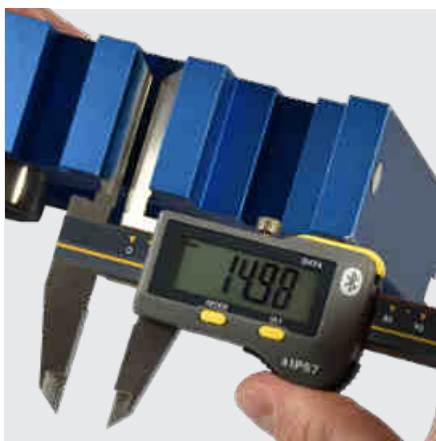
Deep measurement with S_Cal EVO Smart DM
