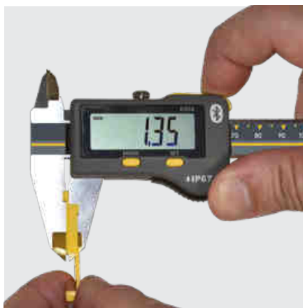
Part measurement with sending data
