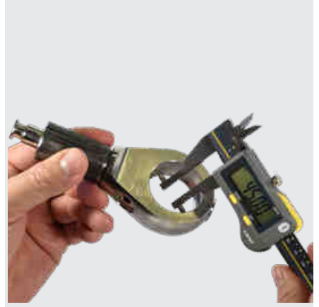
Internal measurement with S_Cal EVO Smart PJ
