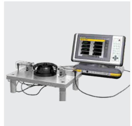
Capacitive probes on a jig
