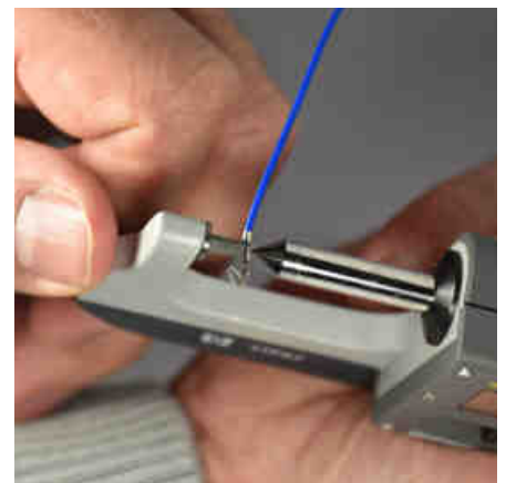
Cable crimping measurement
