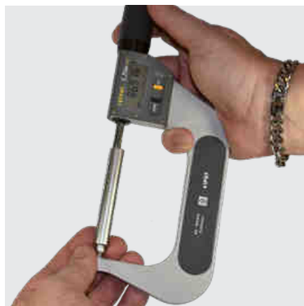
Length measurement of a lathed part
