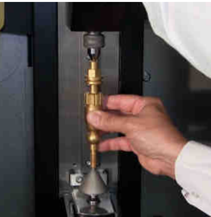
Part measurement with SCAN F60
