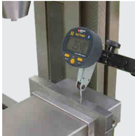
Checking the alignment on milling machine.
