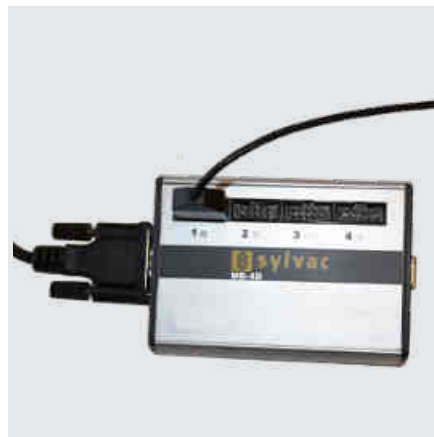
Digimatic instruments connected to a MB-4D
