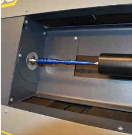
Measurement of a turned part with SCAN 52
