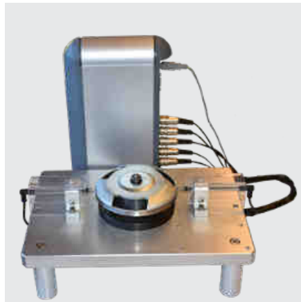
Capacitive probes connected to a D200S.
