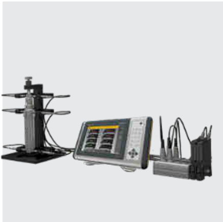
Multiple instruments connection through M-BUS inputs
