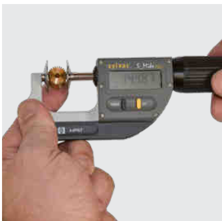
Part measurement with a S_Mike PRO Disk
