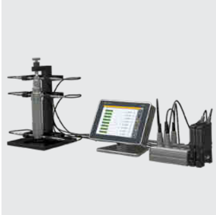
Probes connection through M-BUS inputs
