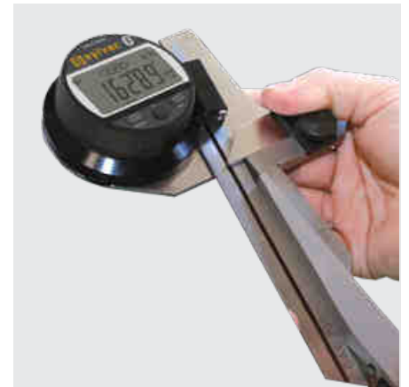
Measurement with accessory type 820-2461
