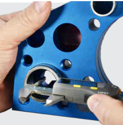
Deep measurement with S_Cal EVO Smart DM
