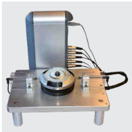
Capacitive probes connected to a D200S
