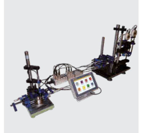
Probes and indicators connection through M-BUS inputs
