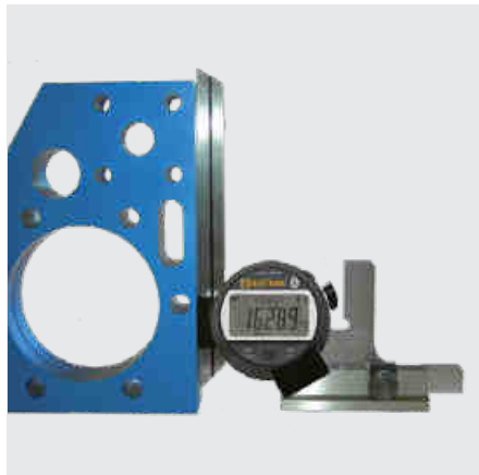
Measurement with accessory type 820-2460
