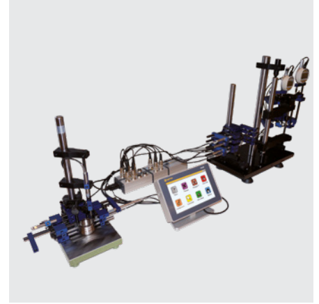
Probes and indicators connection through M-BUS inputs
