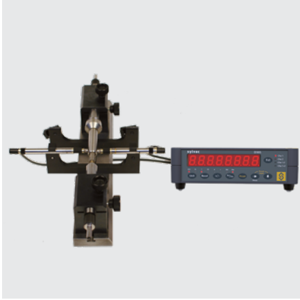
Measuring a shaft with 2 probes (A+B)
