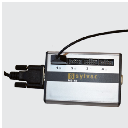
Digital instruments connected to a MB-4D
