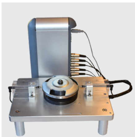
Capacitive probes connected to a D200S.
