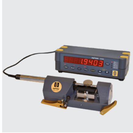
PS15 with connected to a D50S
