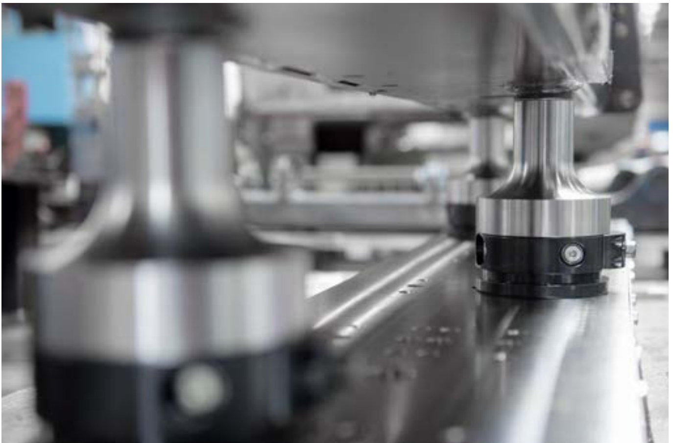
Optimisation of set-up times in small-series production by means of variable, direct clamping of the component. The double clamping modules can be adapted quickly to the different components simply by repositioning.
