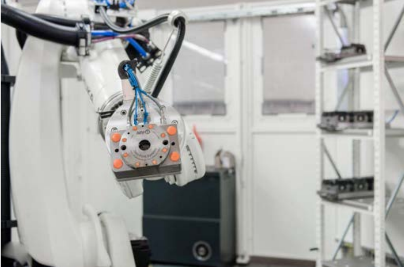
Automation solution with AMF zero-point system as standard interface for robotic loading.
