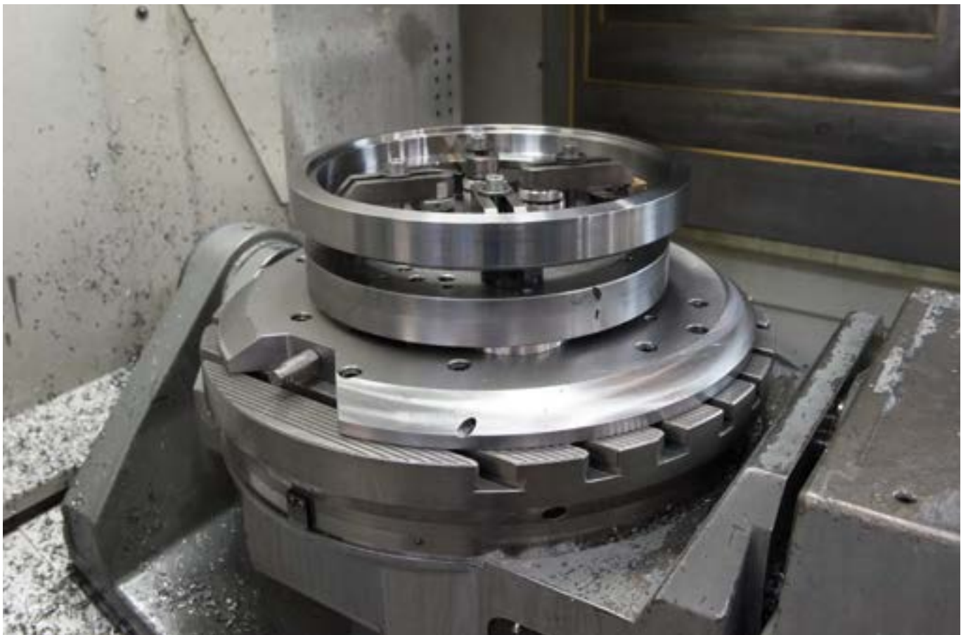
5-axis-machining of machine building components. 4-point clamping station with individual outer contour for maximum accessibility.
