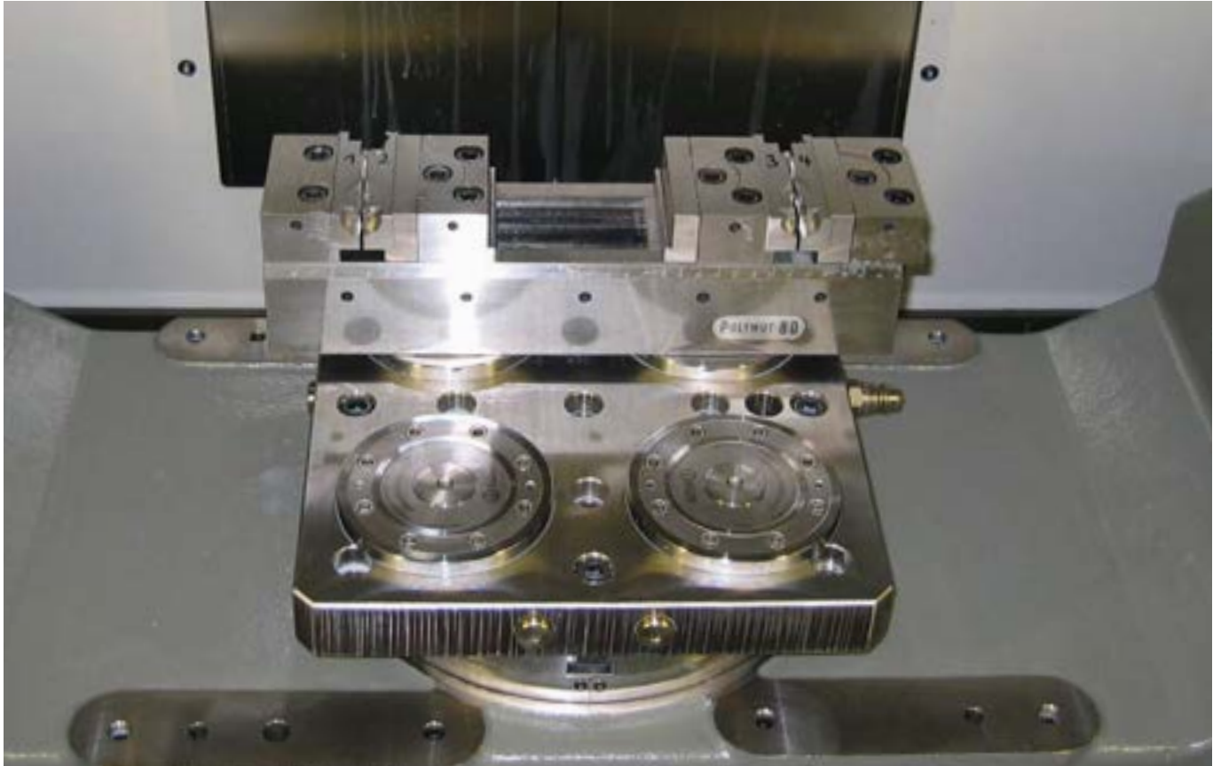
The 4-point clamping station replaces the machine table. This guarantees maximum utilisation of the machine's stroke.
