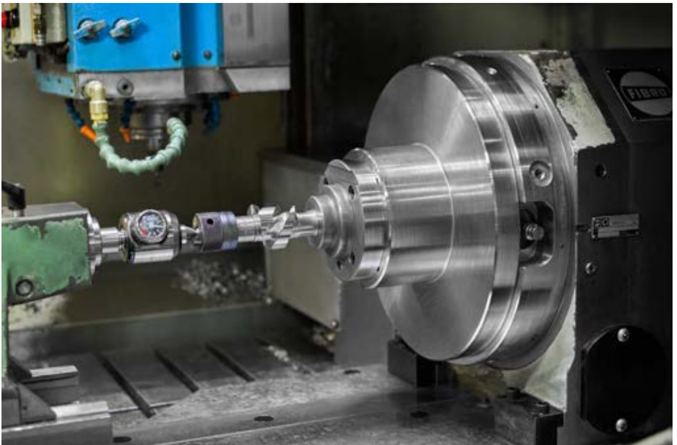
AMF zero point clamping system in use on a grinding/milling machine. It is well worth using, particularly in the case of existing machines with long and frequent set-up procedures.
