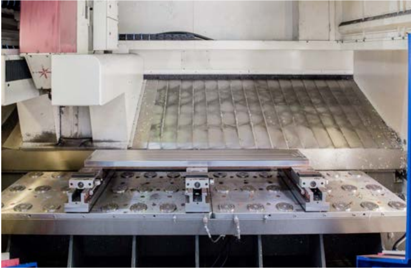
Easy alignment of multiple vices when machining long workpieces.
