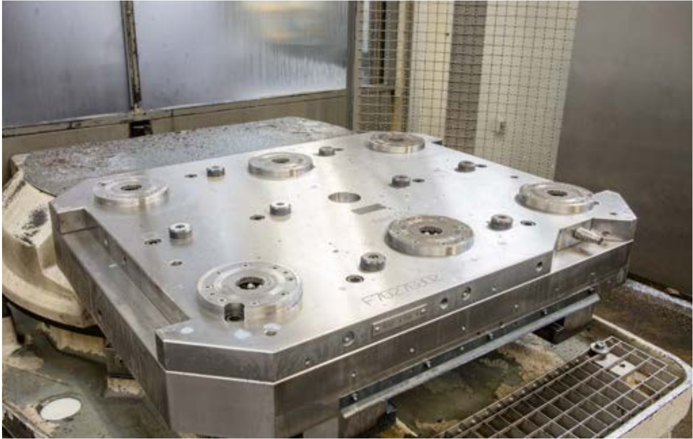
Zero-point clamping technology used in large engine production. Efficiency by setting up mechanical clamping fixtures in parallel during production time.
