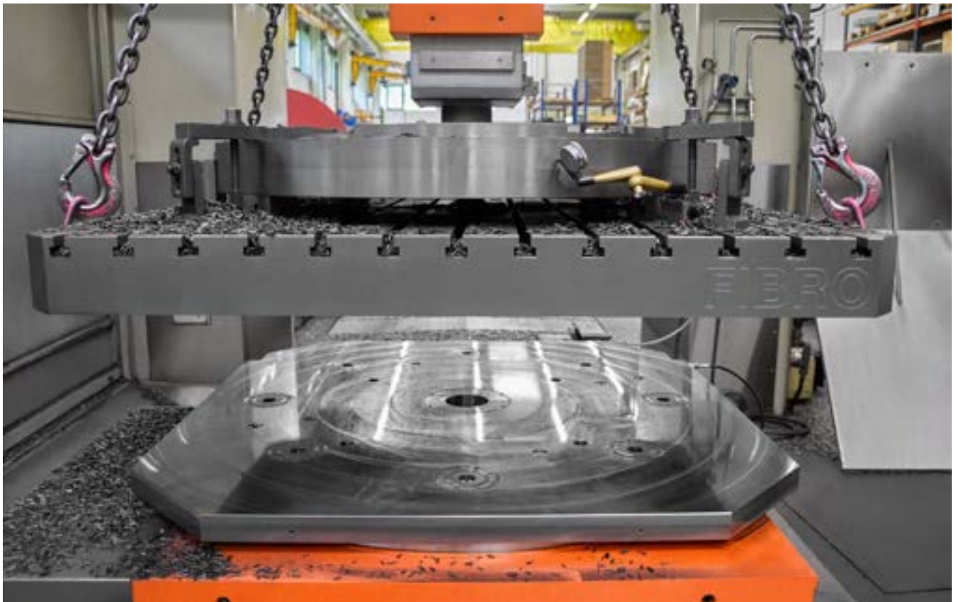
Top and bottom-sided integrated clamping module in a rotary indexing table. The set-up times have been reduced from several hours to a few minutes and the flexibility of the entire machine has been increased to a maximum.
