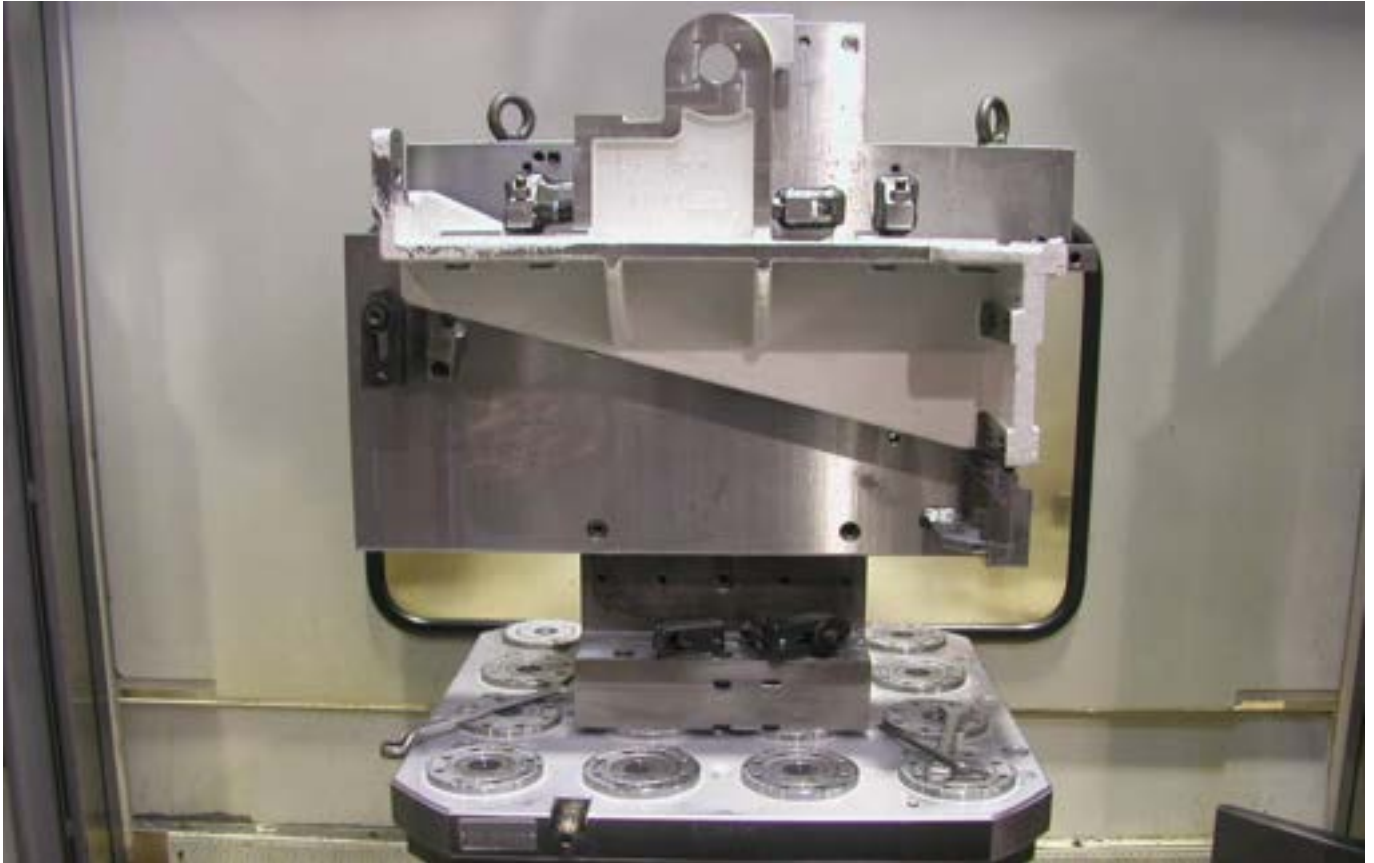
The AMF zero-point system offers a secure fit during drilling operations under unfavourable lever ratios. Thus, even complex workpieces with high cutting parameters can be machined reliably.
