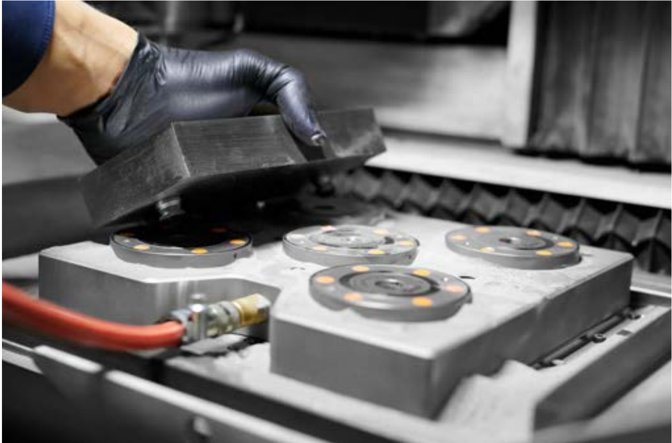
AMF-Zero-Point-Systems in additive manufacturing. The 5-point clamping station enables the substrate plate to be changed quickly on the hybrid machine (SLS / HSM).
