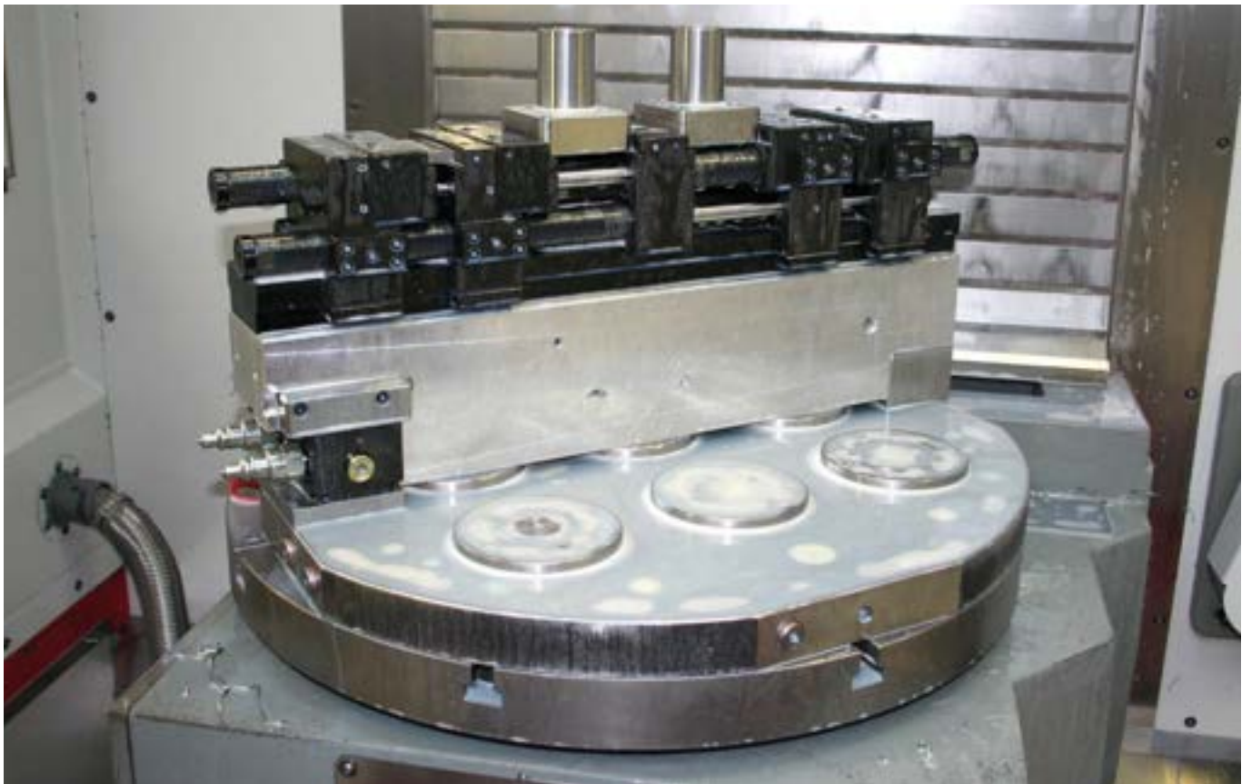
Hydraulic vice for machining multiple or various workpieces in one clamping process clamped on the zero-point system.
