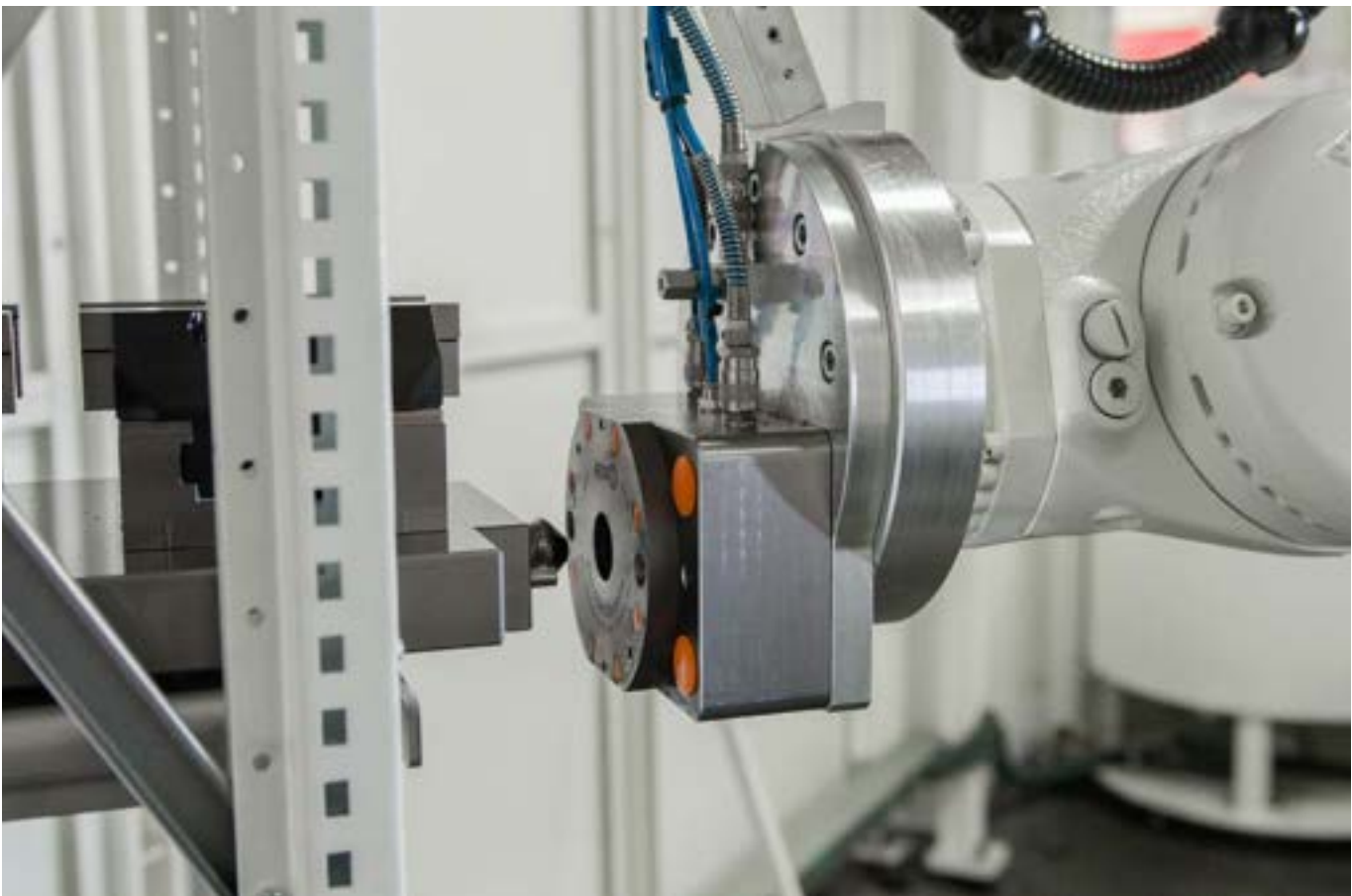
Automation solution with AMF zero-point system as standard interface for robotic loading.
