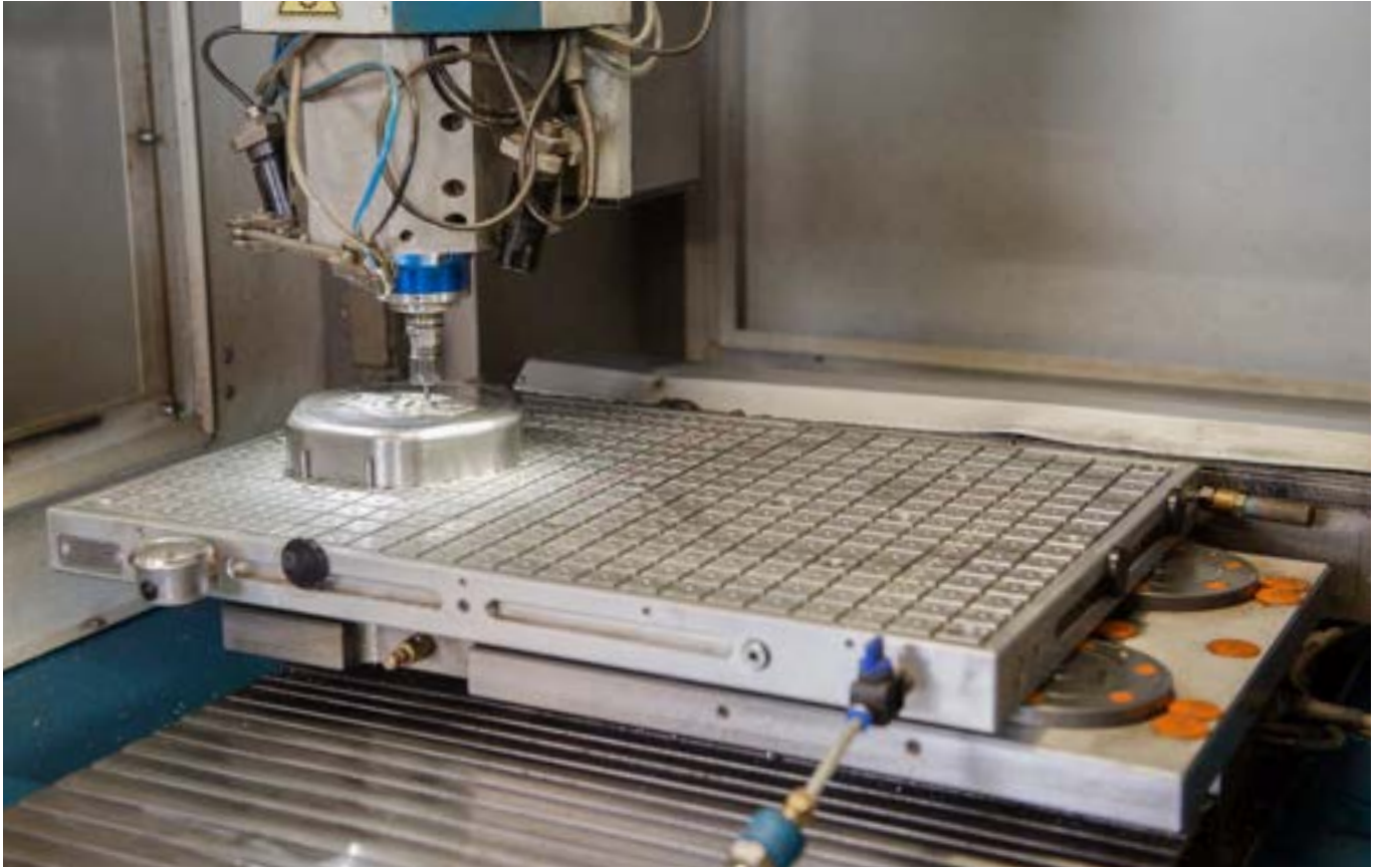
Combined application of vacuum and zero-point clamping technology. The vacuum clamping plate is equipped with pull-stud mountings at the factory.
