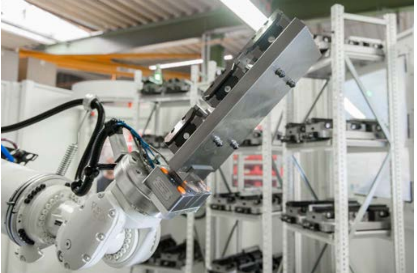
Numerous sensor options and reliable fit with high handling weights guarantee smooth integration into automated robotic loading as well as subsequent machining.
