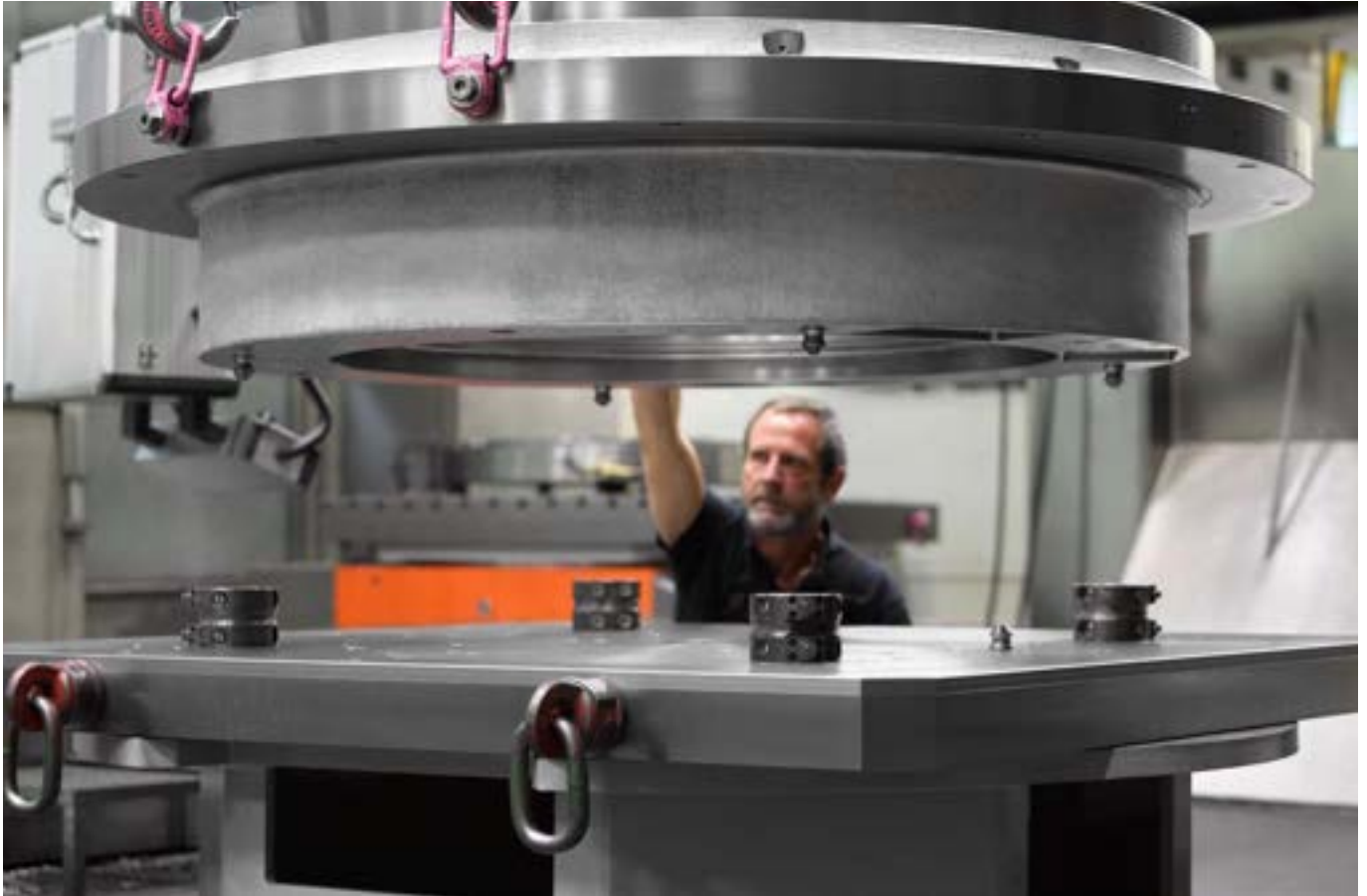
Optimisation of set-up times in small-series production by means of variable, direct clamping of the component. The double clamping modules can be adapted quickly to the different components simply by repositioning.
