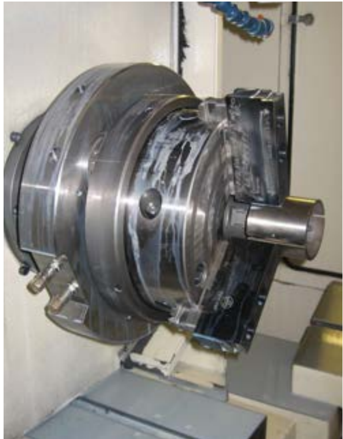
The high precision of the AMF zero-point system permits use in grinding technology.
