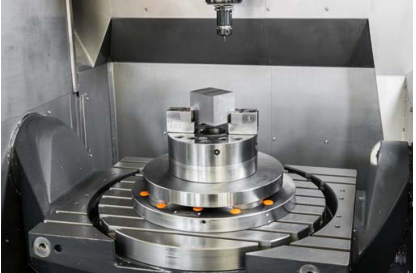
4-point clamping station with integrated bearings and direct locking control system for use on milling-grinding machines up to a maximum speed of 2200 rpm.
