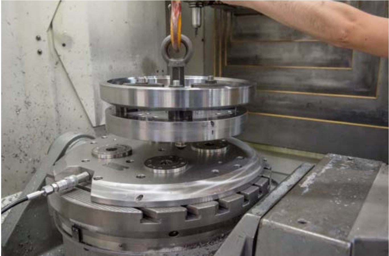
5-axis-machining of machine building components. 4-point clamping station with individual outer contour for maximum accessibility.
