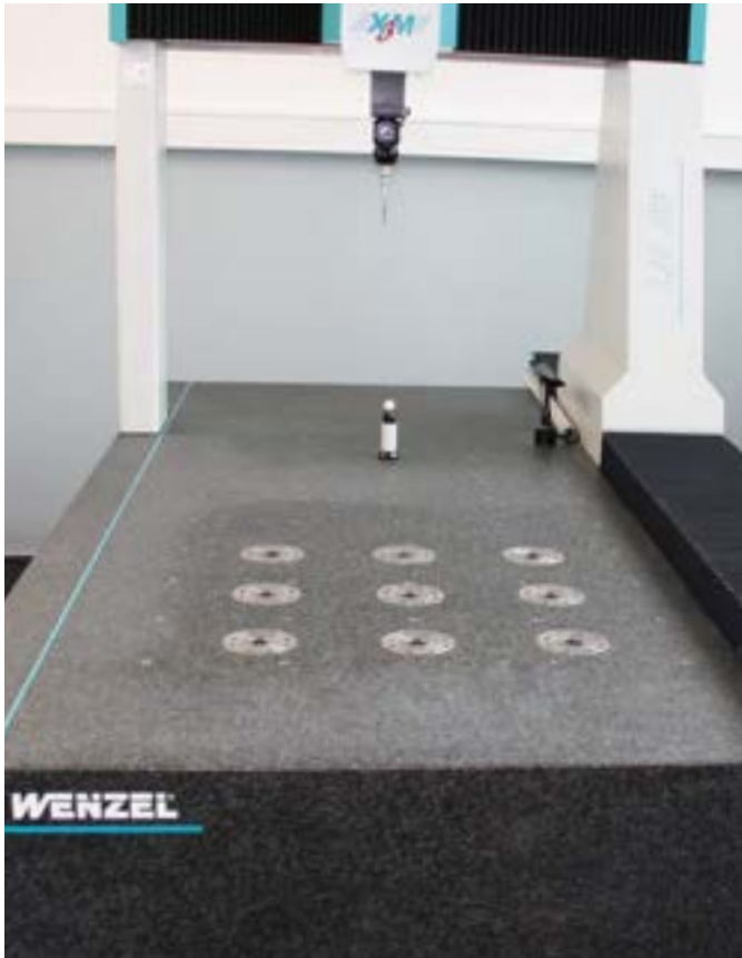
Zero-point clamping technology as standard interface on a coordinate measuring machine. Automation even in post-processing.
