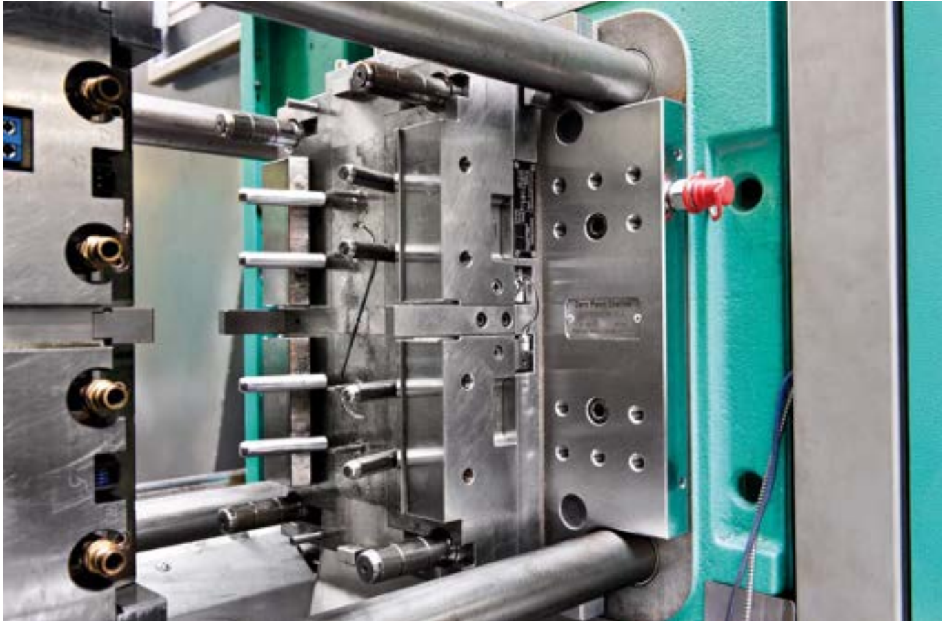
In injection moulding, the tools are successfully changed in a way that optimises set-up time through the use of the AMF zero-point system. With friendly recommendation of Robert Bosch GmbH, Waiblingen
