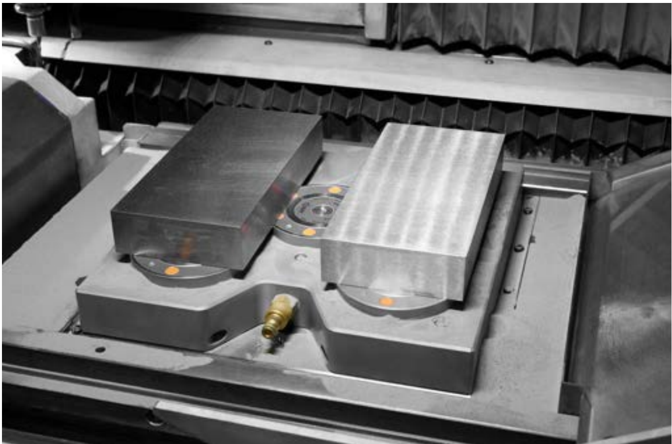
AMF-Zero-Point-Systems in additive manufacturing. The 5-point clamping station enables the substrate plate to be changed quickly on the hybrid machine (SLS / HSM).
