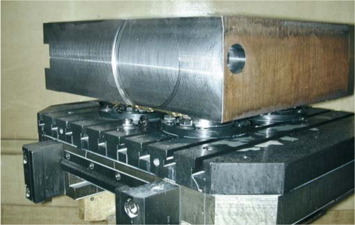
Surface-mounted clamping modules with clamping flanges for easy and flexible positioning of the T-slot tables.
