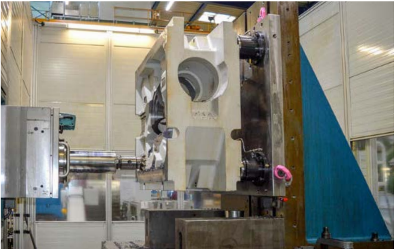
Direct clamping of the workpiece on a horizontal machining centre. Two of the four zero-point clamping consoles can be adjusted in height. This enables workpiece tolerances to be compensated.
