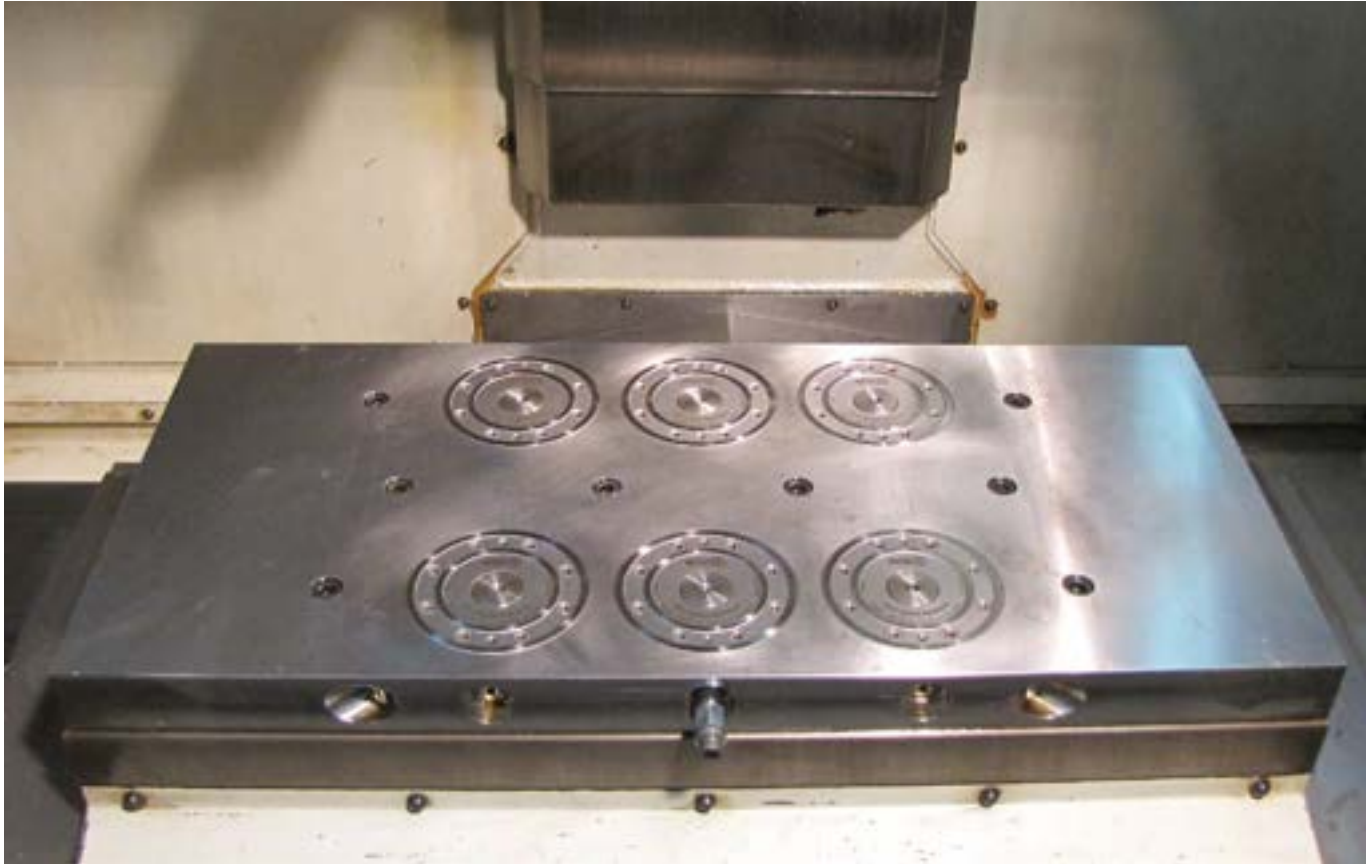
The cylindrical mating receptacle makes recessed installation of the clamping modules easily possible without any loss of precision.
