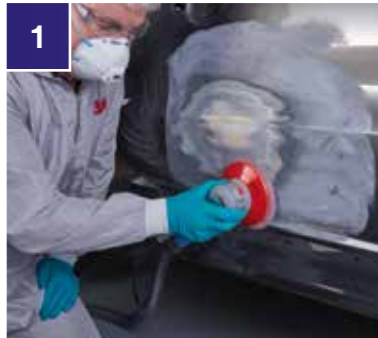
1 Further key around the repair area using 3M™ abrasive discs, grade P320 and P500.
