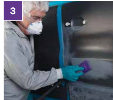
3 Hand block or machine sand the repair area using P320 3M™ Hookit™ Abrasive Sheets.
