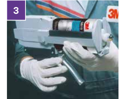
3 Place duo pack cartridge with adhesive in applicator. Unscrew adhesive cap and dispense enough to equalise the adhesive. Attach and lock the mixing nozzle to the duo pack cartridge.
