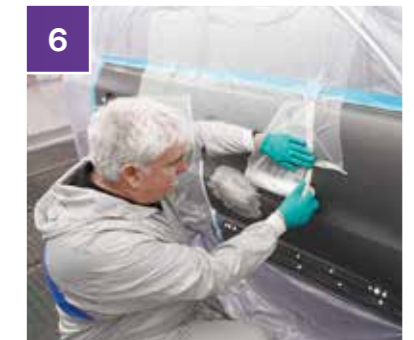
6 Use appropriately sized 3M™ Pre-taped Masking Film to speed up masking operations and for SMART repairs.
