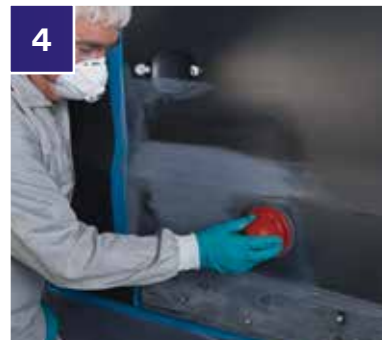
4 Reapply 3M™ Dry Guide Coat to the panel.
