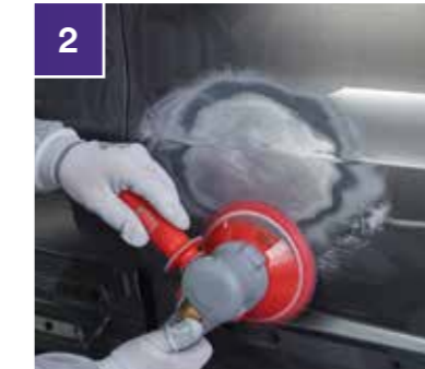
2 Remove paint from damaged area using a dual action sander with relevant 3M™ abrasive ranging from P80 to P120.
