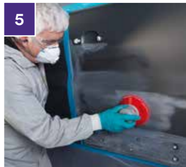
5 Machine sand using fine grade abrasives P400 or P500.
