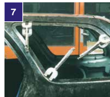
7 Spray 3M™ Weld Thru II Coating (50410) to all areas to be welded. Clamp the panel in its proper position.
