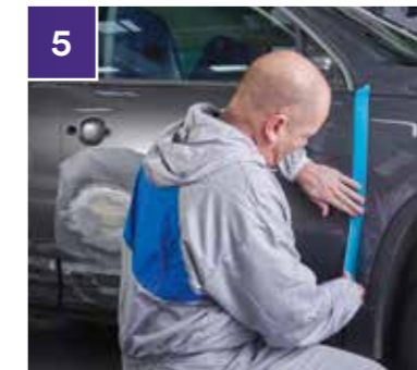
5 Use 3M™ Scotch® Performance Masking Tape for critical areas and for general masking.
