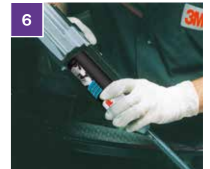
6 Apply additional adhesive bead to either the replacement panel or the inner structure.
