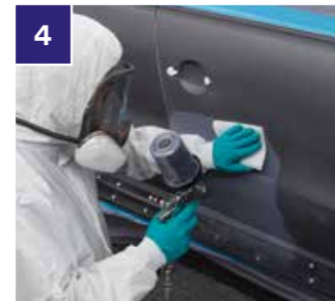
4 Check all masking and tack repair area in preparation for topcoat.
