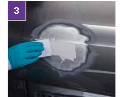
3 Reshape panel as required. Mix and apply body filler to damaged area, avoiding surrounding paintwork.
