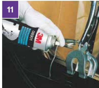
11 Clamps can be removed after 4 hours at 23°C and/or if there is any tension, part needs to remain clamped longer. Curing time may be accelerated by applying heat with applicator or IR lamps (do not exceed 120°C for 45 minutes). Allow 24 hours curing before returning the vehicle to service.
