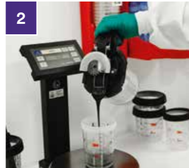
2 Measure out paint accordingly for the job.
