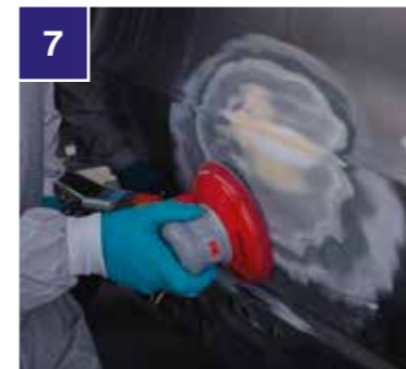
7 Feather around the repair area ensuring that any deep scratches are removed using finer grade abrasives P180.
