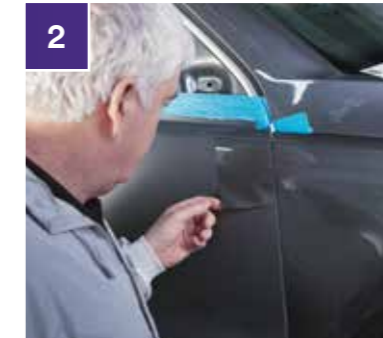
2 Check colour match film spray out against vehicle.
