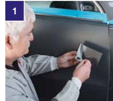
1 Mix small amount of paint and generate a spray out card using 3M™ PPS™ Colour Match Film.
