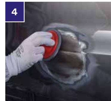
4 Apply 3M™ Dry Guide Coat and hand or machine sand the filler to the desired shape.
