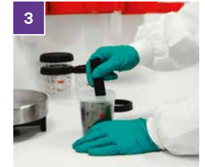
3 Mix colour in 3M™ PPS™ Liner, selecting the appropriate size for repair area.
