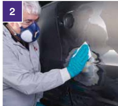
2 Blow and wipe down with degreaser using 3M™ Professional Panel Wipes.
