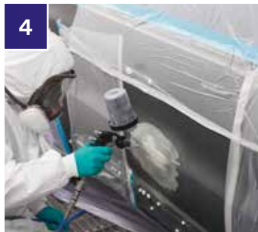
4 Apply etch primer on any bare metal areas using 3M™ Accuspray Gun and 1.4mm nozzle.
