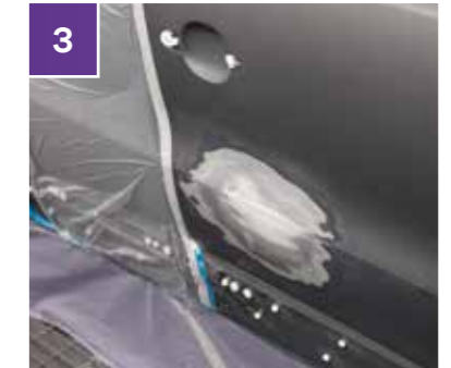
3 Use 3M™ Soft Edge Masking Foam tapes for standard aperture masking requirements. Foam tape can also be used to fill voids where trim had been previously attached.
