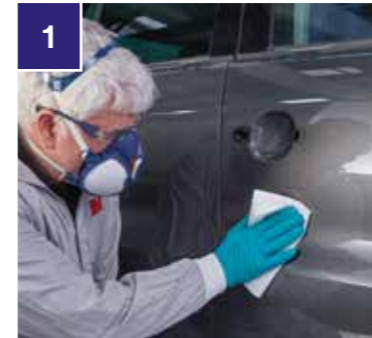
1 Inspect the damaged area and degrease in accordance with paint company recommendations.
