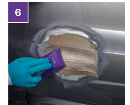
6 Apply 3M™ Dry Guide Coat and hand sand the filler or glaze to the required shape and finish using (finer grade abrasive) P180 abrasive.
