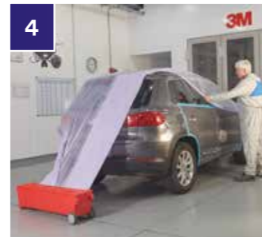
4 Use 3M™ Masking Film to protect those large areas of the car not to be sprayed during the repair.
