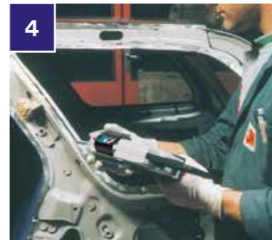
4 Apply adhesive bead on all areas to be bonded (all bare metal surfaces).
