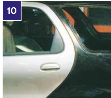
10 Spray the inside quarter panel and weld the seams with 3M™ Inner Cavity Wax, Amber (08901) or Transparent (08909).
