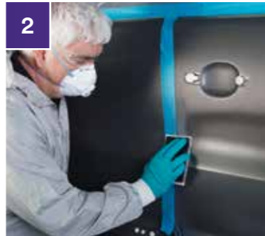
2 Hand sand awkward primed areas and panel edges using 3M™ Hookit™ Flexible Abrasive Sheets or 3M™ alternative.
