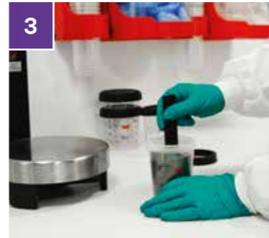
3 Use a 3M™ PPS™ Mixing Stick to stir the paint thoroughly.
