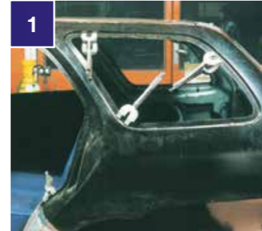
1 Remove all paint, rust and contamination from surfaces to be bonded using 3M™ Roloc™ Bristle or Clean and Strip™ Discs. Straighten all metal, clamp the part in place and check for fit alignment.
