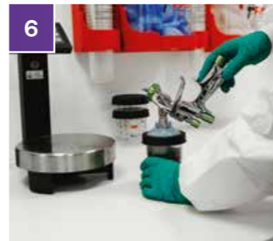
6 Upon completion of spraying, invert the gun and pull the trigger to return paint to 3M™ PPS™ before disconnecting. Dispose of the 3M™ PPS™ Lid/Liner and clean the gun and adapter.
