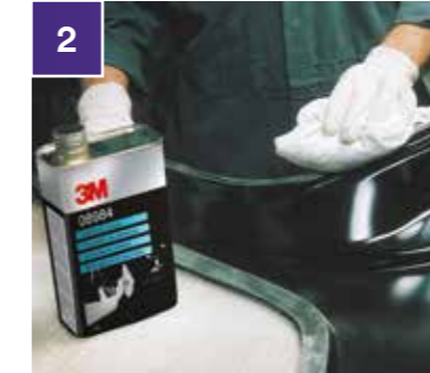
2 Clean all areas to be bonded with 3M™ General Purpose Adhesive Cleaner (08984).
