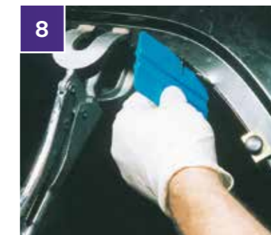
8 Tool out any 'squeezed out' adhesive to seal the outside of the seam all along the bonded edge of the panel.
