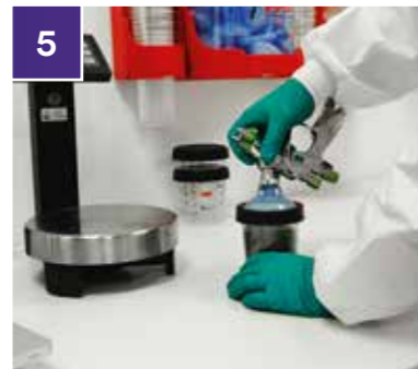
5 Attach 3M™ PPS™ to gun by aligning the 3M™ PPS™ Lid Legs with the PPS™ adapter and then twist to lock.
