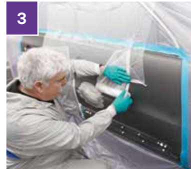
3 Apply the appropriate 3M™ masking products to suit the repair area and move vehicle into the booth.
