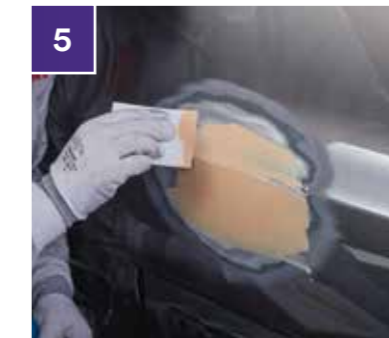
5 Assess the filled area and apply additional fillers or 3M™ Premium Glaze as required.
