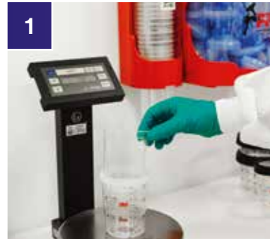
1 Place 3M™ PPS™ Liner inside a 3M™ PPS™ Cup on paint mixing scales at zero.
