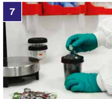
7 To store colours for future use, insert a sealing cap in the top of the 3M™ PPS™ Lid.
