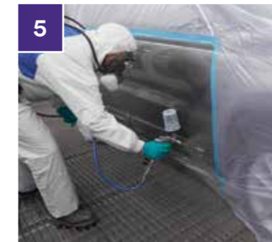
5 Apply paint and bake as per paint company recommendations.
