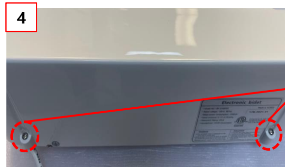
④ Screw the 2 screws back using a Phillips head driver.
