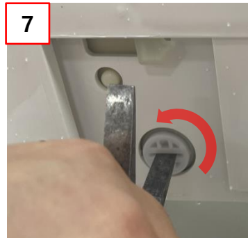
7 Cap drain groove (13mm*2mm) Please use coin or flat screwdriver to unscrew the cap
