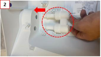
2) Attach the DAMPER to the SEAT and SEAT COVER
