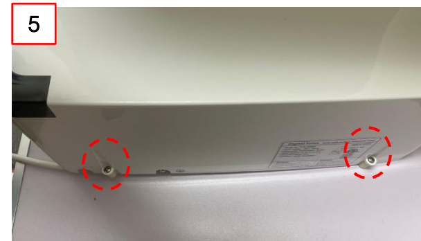
⑤ Screw the 2 screws back using a Phillips head driver.
