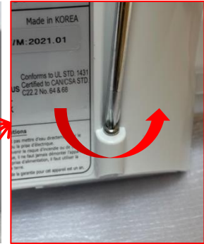
③ Unscrew the 2 screws at the back using a Philips head driver.
