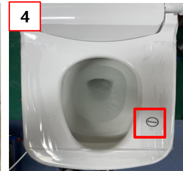
Check the seat sensor label position.
