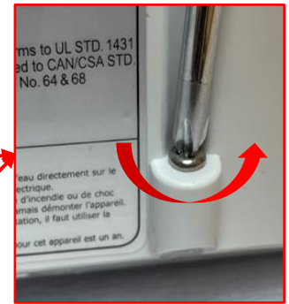
③ Use a screwdriver to remove 2 screws at the back.
