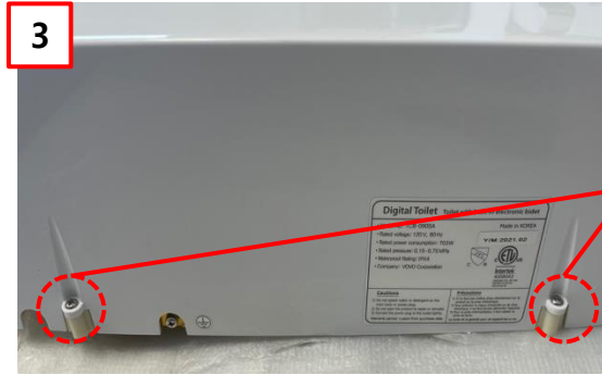
③ Unscrew the 2 screws at the back using a Philips head driver.
