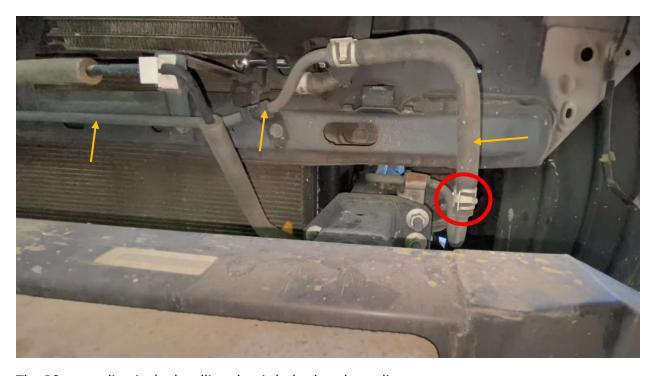
The PS return line is the hardline that is bolted to the radiator support.
