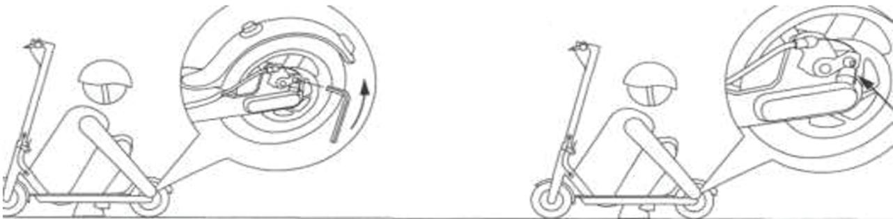
If you feel the brakes are too tight, please use the M5 hex wrench counterclockwise to release the pressure plate screws on the disc brake seat, return the brake line to make the exposed tail length slightly shorter, and lock the pressure plate screws; If you feel the brake is too loose, release the pressure plate screws, drag the brake cable to make the exposed tail length slightly longer, and then lock the pressure plate screws.
