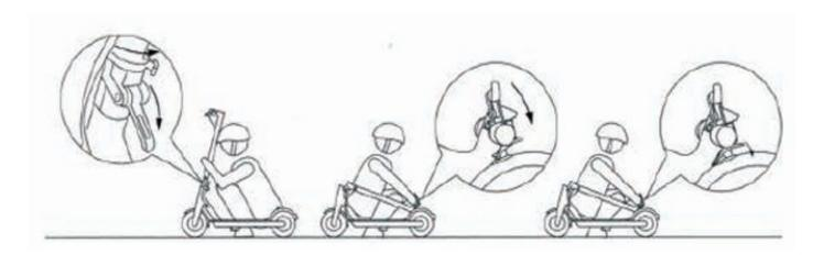
Make sure the electric scooter is turned off and from the vertical tube take out the folding wrench, fold the tube towards the rear wheel.
