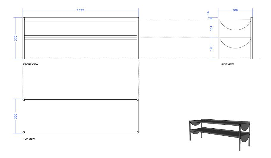
Mouse Shoe Rack Technical Drawing Scale 1:10 Unit: mm
