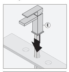
1b) SLS3612: Insert faucet body (E) through deck plate (Z) and deck surface.
