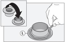
5) Push Pop Install: Insert drain body (L) into drain opening. From below, Tighten locking nut (O) with gasket (M) and washer (N) to flange. Tighten tail nut (Y) with washer (X) to secure tail pipe (Q).
