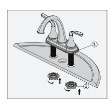
2) Make connections to water lines. Use 1/2" IPS faucet connections (1)or use the supplied coupling nuts (3) with 3/8" O.D. ball-nose risers (2).Use wrenches to tighten connections.
