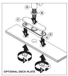
5) Secure Faucet Mounting Hardware: From below deck, slide plastic washer (B) and metal washer (C) onto threaded faucet body (A)...
