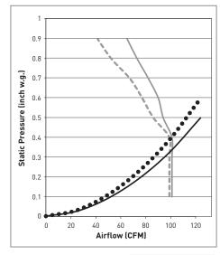
Net Supply Air Net Exhaust Air • • • 4" 60ft Duct 4" 70 ft Duct
