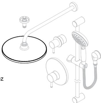
Locate the component box with SKU label **1660730** and install the **Shower Slide Bar**
