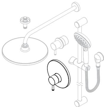
Locate the component box with SKU label **T064430** and install the **Diverter Trim**
