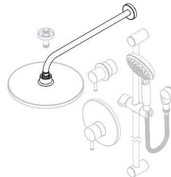
Locate the component box with SKU label **1695001** and install the **11in Rain Shower Head**
