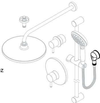
Locate the component box with SKU label **8888035** and install the **60in Metal Shower Hose**
