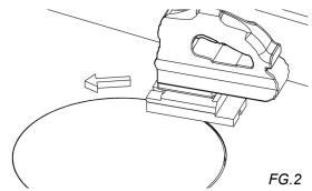
2. Cut out the counter -The cutting tools required will depend on the surface to be cut. FG.2 (Your sink comes with 4 mounting screws for mechanical fastening. Screws are only necessary if for some reason silicone cannot be used. In this case, you will need to drill 4 holes in the counter to accommodate these screws)
