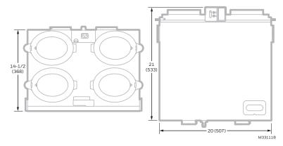
Fig. 1. Dimensions in in. (mm) and clearances.
