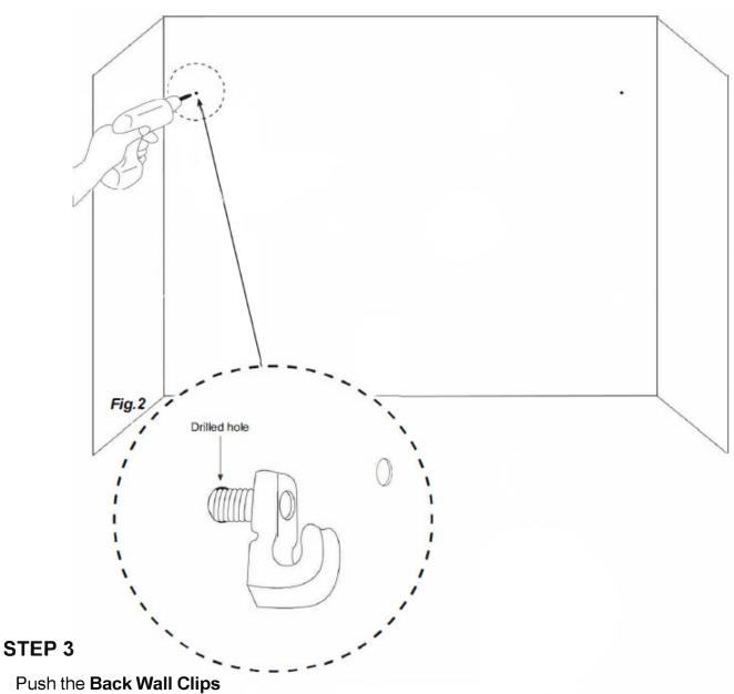
Push the **Back Wall Clips** half way into the holes as in **Fig 2**.
