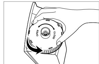
3. Put in water and turn the water tank cap in a clockwise direction until you hear a click as it locks.
