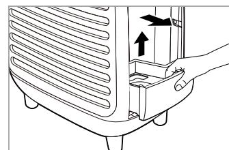
2. Carefully remove the humidifying filter so water doesn't splash, and then replace it.
