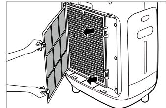
3. Remove dust with water or a vacuum cleaner depending on the degree of contamination.
