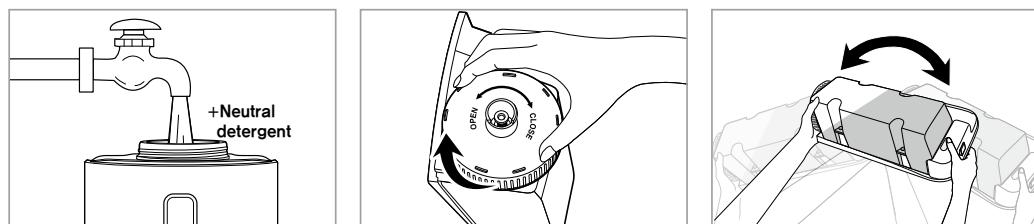
3. Turn the water tank cover in a counter-clockwise direction to open and discard the water mixed with detergent, then rinse well in running water.washed.
