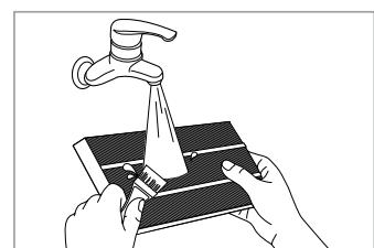
3. Remove the humidifying filter, shield, and cistern cover from the cistern in order and then wet a soft cloth or cleaning brush in neutral detergent and wipe the cistern under running water. Wipe away moisture from the cistern with a soft, dry cloth and dry in a shady place.
