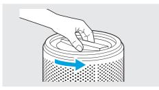
Grab the handle and turn clockwise to close and turn counter clockwise to open the rear cover.
