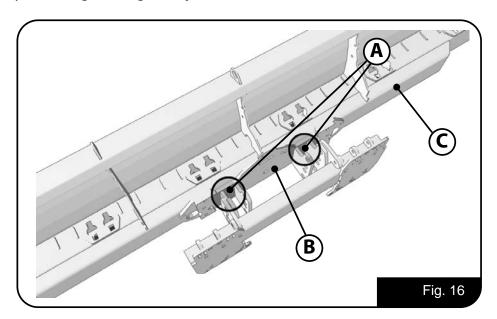
Find the two(2) greasing points  $\bf A$  located behind the blade/plow, the two(2) greasing points are located on the plate  $\bf B$ , itself bonded to the main beam  $\bf C$ , as shown Fig. 16.
