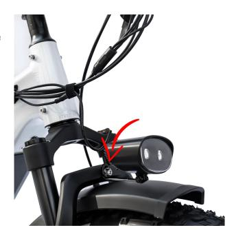
STEP 7: Place the front rack into position aligning with the mounting points on the head. The brake lines should go in between the opening of the front rack.
