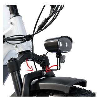
STEP 1: Unplug the headlight connector. Snip zip ties as needed, then pull each side of the connector directly apart, without twisting, to unplug.
