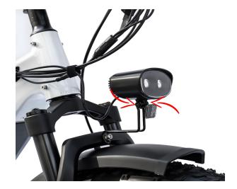
STEP 3: Using a 5 mm allen wrench and a 10 mm wrench loosen the bolt that holds the headlight mount to the front forks. Remove the stock mount.
