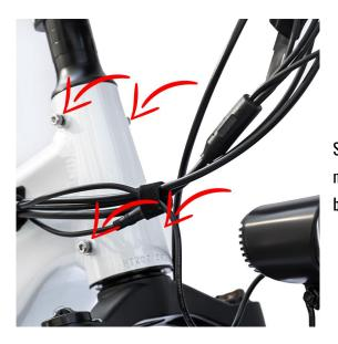
STEP 8: Using the bolts removed in step 6, use a 4 mm allen wrench to tighten them onto the mounting tabs. You should have room to make small adjustments up or down. Tighten but do not over tighten.
